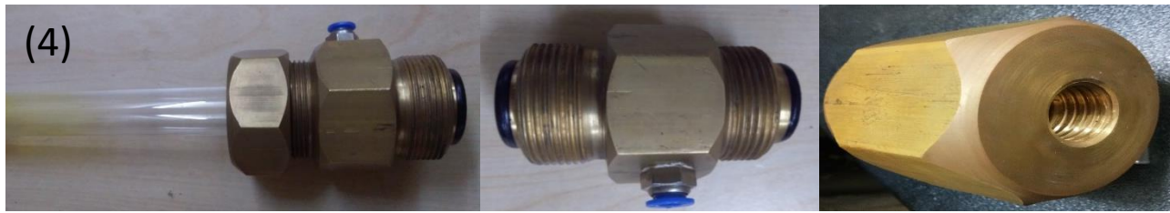
Fig-4. Typical gas tight flange arrangement to be used in different joints.
